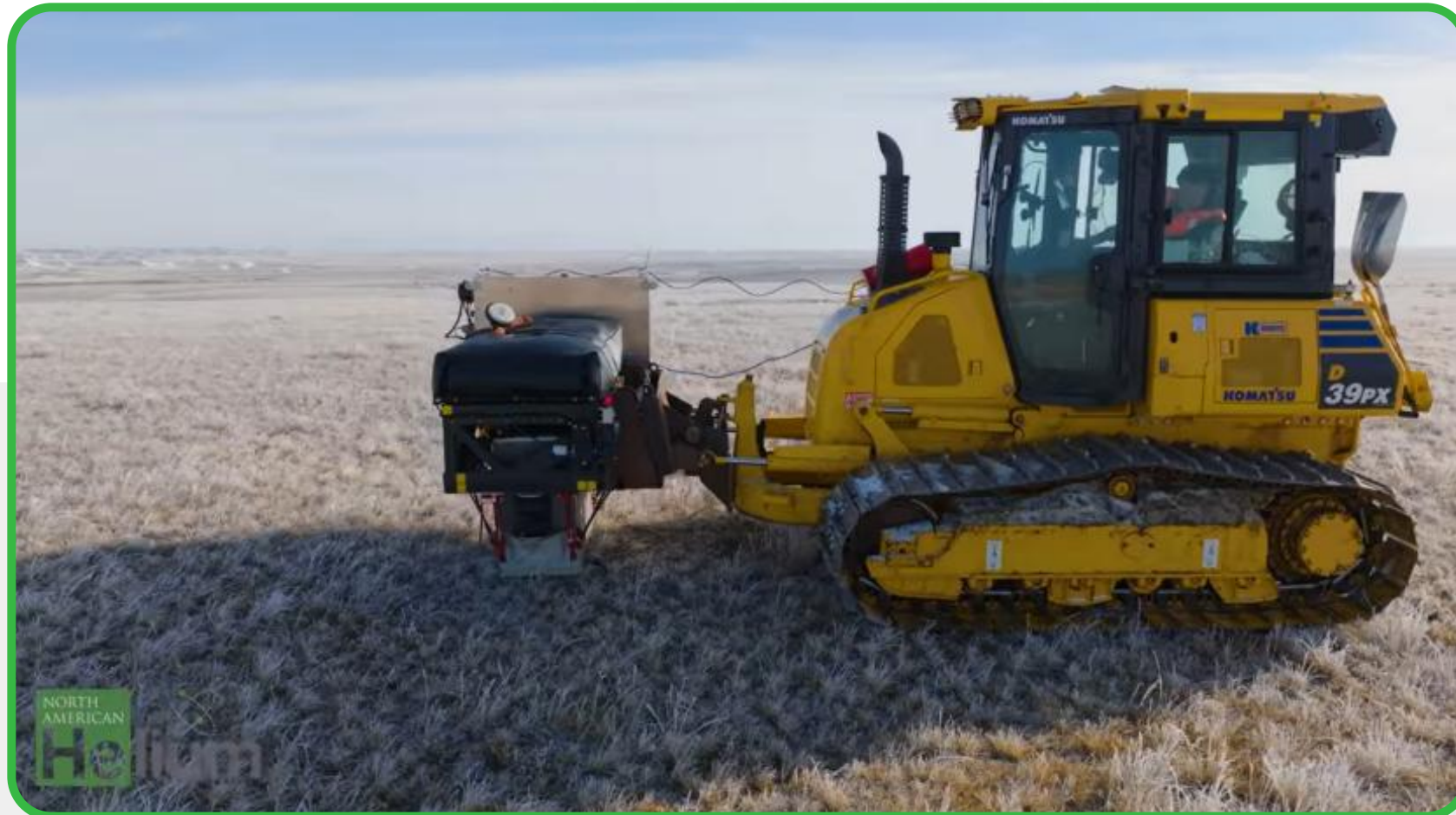
Source: NAH; eVibe seismic unit – minimal environmental disturbance
